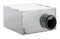
• Casing and motor-support made of galvanized sheet steel; lined internally with PE sound-proof panel (thickness 10 mm).
